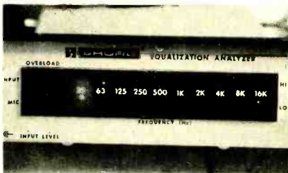
FIG. 8—EQUALIZATION ANALYZER shows total frequency response of hi-fi system after equalization.
