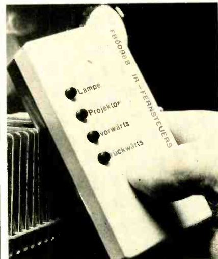
NEW INFRARED REMOTE CONTROL. Channels are Lampe (electric light for room illumination) Projektor , Forward and Back .
